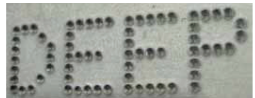
Deep mark with BenchDot™ DP series machine
