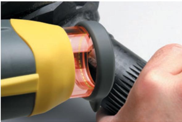
*The DataMan 6500 ID reader is ideally suited for reading very low contrast Data Matrix codes on automotive powertrain, aerospace, and DoD components and assemblies.*
