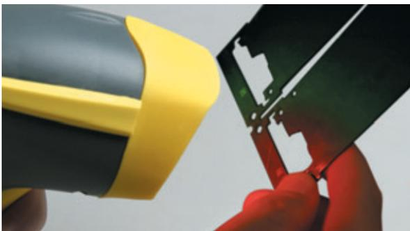
*Electronics manufacturers moving from barcode labels to Data Matrix due to space constraints use DataMan handheld readers for identifying boards and components.*
