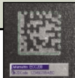
2D Data Matrix code direct-marked on automotive part.
